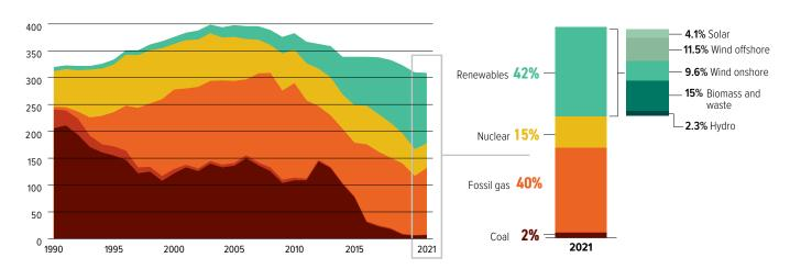
The UK generated 43% of its electricity from fossil fuels in 2021, mainly from fossil gas, but with minimal amounts of coal (2.3%) and oil (0,39%). The share of renewable energy in the UK's power sector has been increasing rapidly, providing around 42% in 2021, up from 13% a decade ago. Wind and solar alone produced 25% of all electricity generated. Renewables have displaced coal from the power sector.
